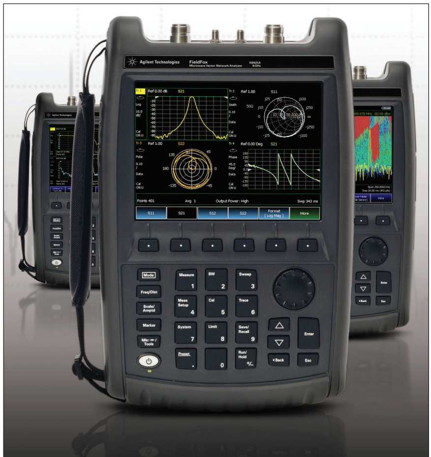
Photo 1: Agilent's FieldFox combination microwave analyzer's base function is a cable and antenna analyzer, and it can be configured to include spectrum and network analysis. Offering amplitude accuracy of \pm 0.5 dB at power-up with no warm-up required, a frequency range up to 26.5 GHz, built-in calibration capabilities and ruggedized operation, the analyzer is suitable for a range of applications including satellite communications, microwave backhaul and military communications.
